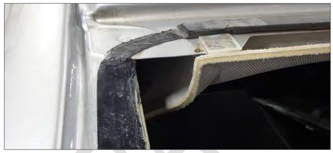
Pinchweld Inspection and Preparation: Close-cut the original urethane down to a thickness of 1 mm - 2 mm. Clean with water and dry with a clean cloth. Apply pinchweld primer to any bare metal scratches if necessary and allow to dry for 10 - 15 minutes.
