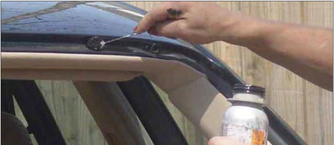
Image 6: Note that windscreen primer must not be applied over any existing cured urethane, or used on large bare metal areas. Windscreen primer must be allowed to dry - typically requiring 10 to 15 minutes - before the application of urethane.
