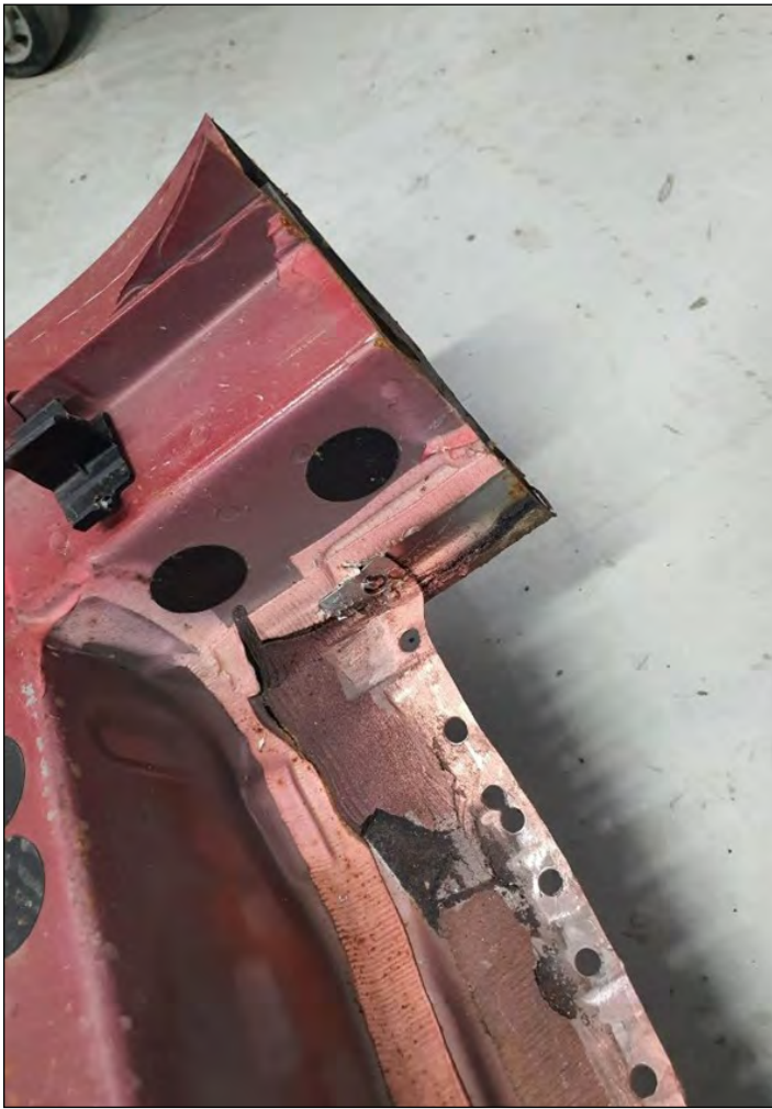
Image 2: Sill and floor join.
