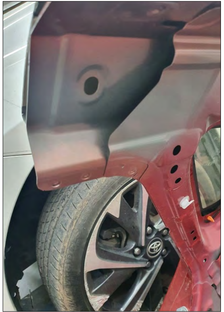
Image 3: Upper pillar and cant rail joins.
